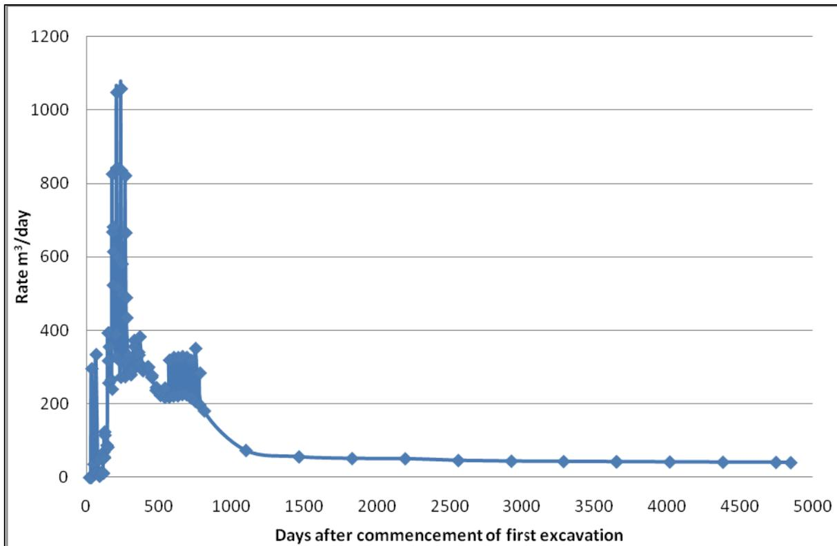
Figure 12-5 Estimated daily groundwater inflows into the entire tunnel system
